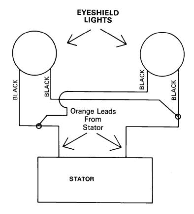
EYESHIELD LIGHT VOLTAGE IS OBTAINED FROM A SEPARATE ISOLATED COIL IN THE STATOR.
